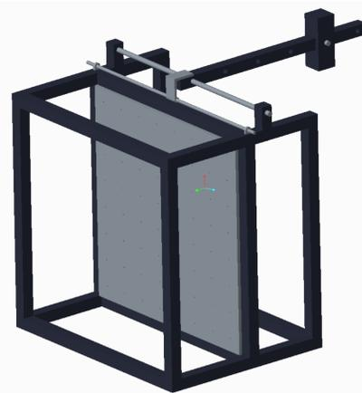
Figure 3 – Solid CAD model of shock test apparatus
