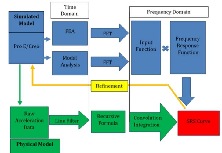
Figure 5 – Data flow for shock testing to SRS curve generation
