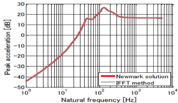
Figure 1 – Example SRS curve, logarithmic scale
